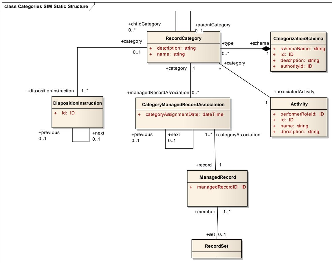
The Categories SIM Static Structure diagram shows the information elements that comprise parameters or information that the Categories service must manage.
