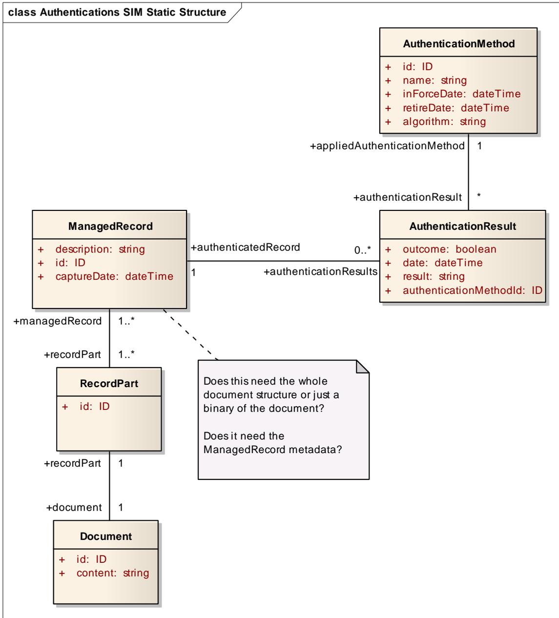
The Authentications SIM Static Structure diagram shows the information elements related to Authentications that this service must manage or use in referencing information managed by other services.
