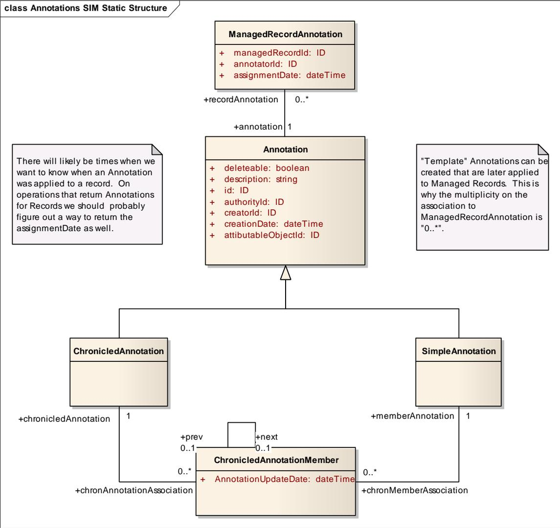
The Annotations SIM Static Structure diagram shows the information elements that comprise parameters or information that the Annotations service must manage.
