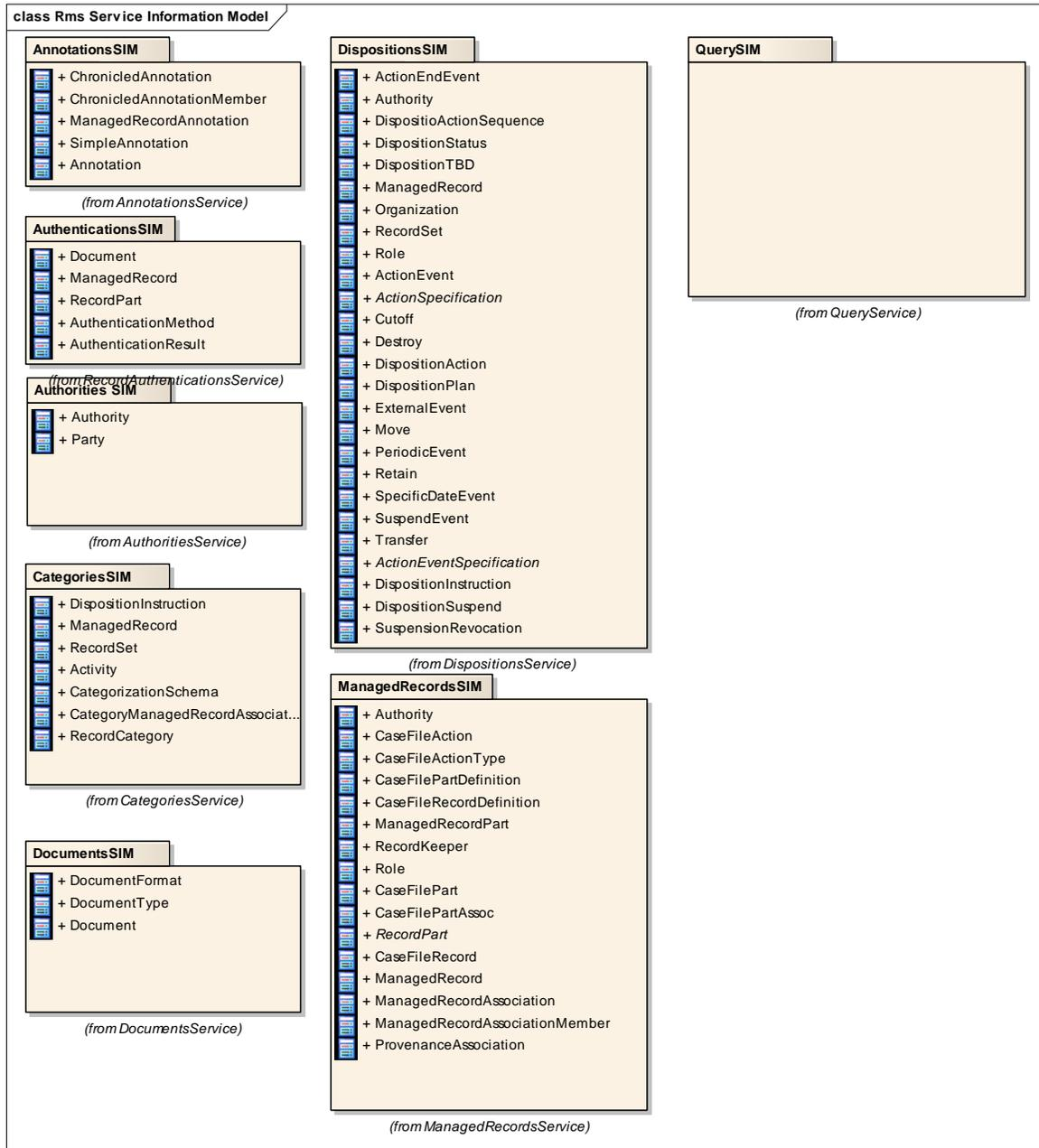
This diagram shows the various Service Information Model (SIM) packages that support the RMS Core Business Services. Each package is contained within the package that defines the associated service. They are included here to facilitate understanding of the information elements contained throughout these services.
