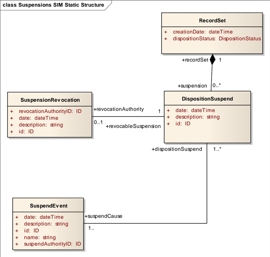
The Suspensions SIM Static Structure diagram shows the information elements related to the suspension of managed record dispositions and the corresponding suspension revocations that the Dispositions service must manage.
