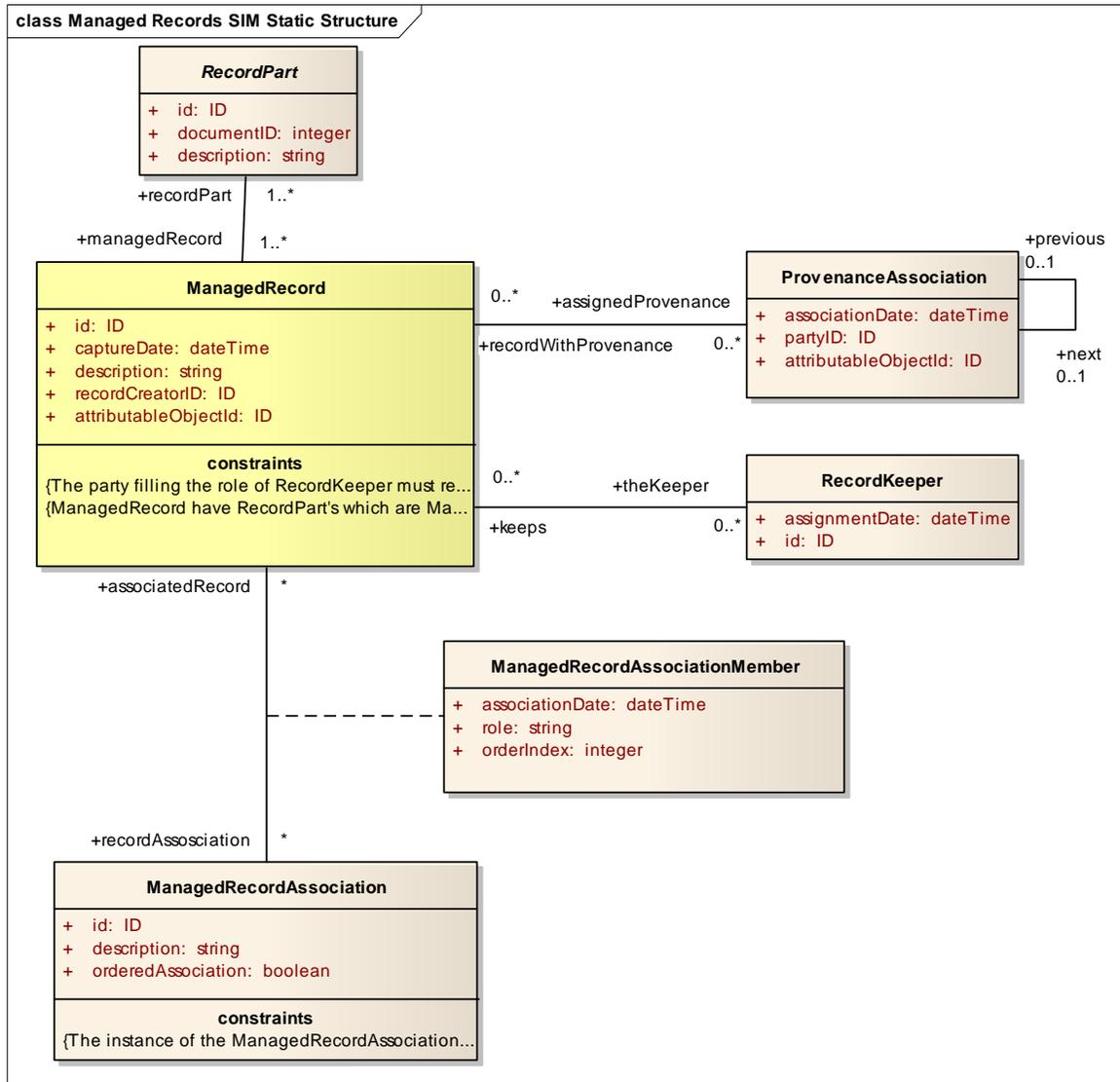
The Managed Records SIM Static Structure diagram shows the information elements related to Managed Records that this service must manager use in referencing information managed by other services.
