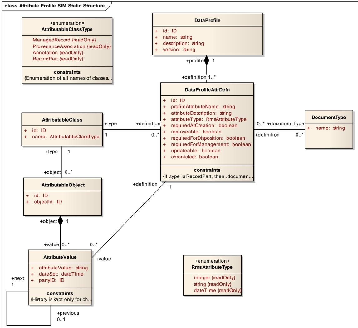
The AttributeProfile Service SIM Static Structure diagram shows the information elements that comprise parameters or information that the AttributeProfile service must manage.
