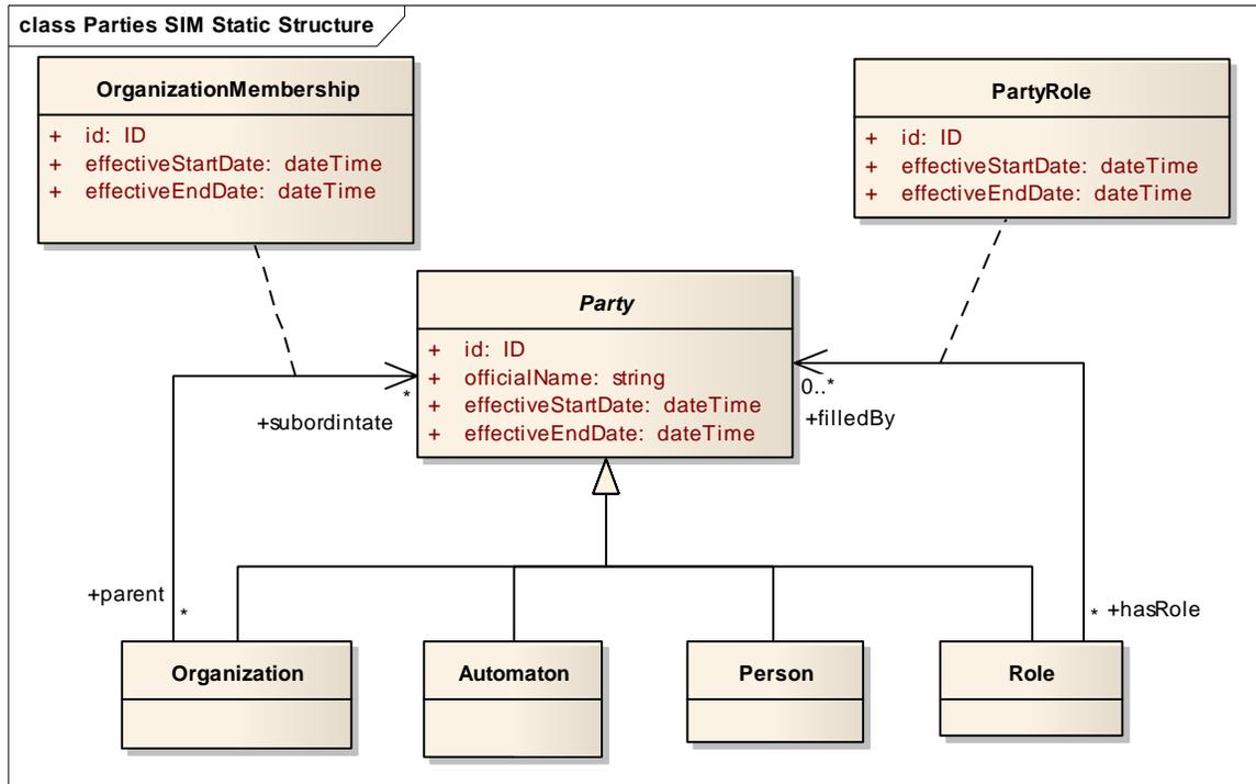
The Parties Service SIM Static Structure diagram shows the information elements that comprise parameters or information that the Parties Service service must manage.
